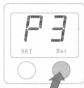
Capacity of battery is shown on the Nixie tube
